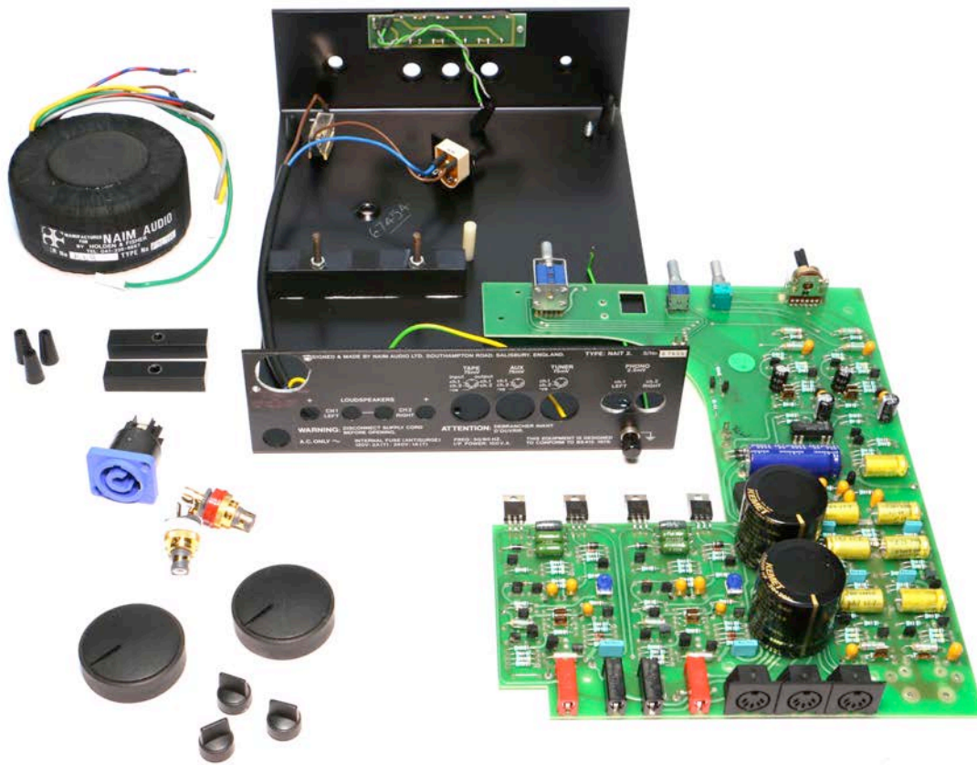
Parts ready for reassembly in an AVO Ultimate Upgrade NAIT2 ... including rebuilt circuit board, Deep-Cryo'd transformer, PowerCon connector and WBT RCA sockets.
