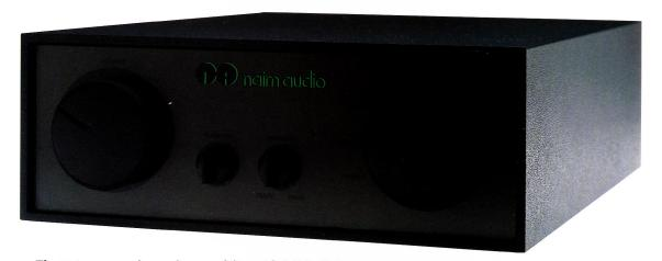
The 72 is a more advanced preamplifier with full facilities – two tape inputs, tape monitor, tuner, and two fully convertible inputs for phono, CD or other ancillary equipment. New enhanced circuitry includes a matched and time-aligned filter. On turn-on, output to the amp is delayed until normal operating conditions have been reached.
