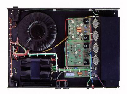
Both these amplifiers use very large high quality toroidal transformers. Power transformer design is a very specialised field and our transformers are the result of many years of closely co-operative development with our manufacturers. The 250 has four regulated power supplies each of
